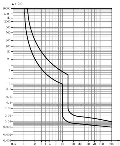
D type protection characteristic curve
